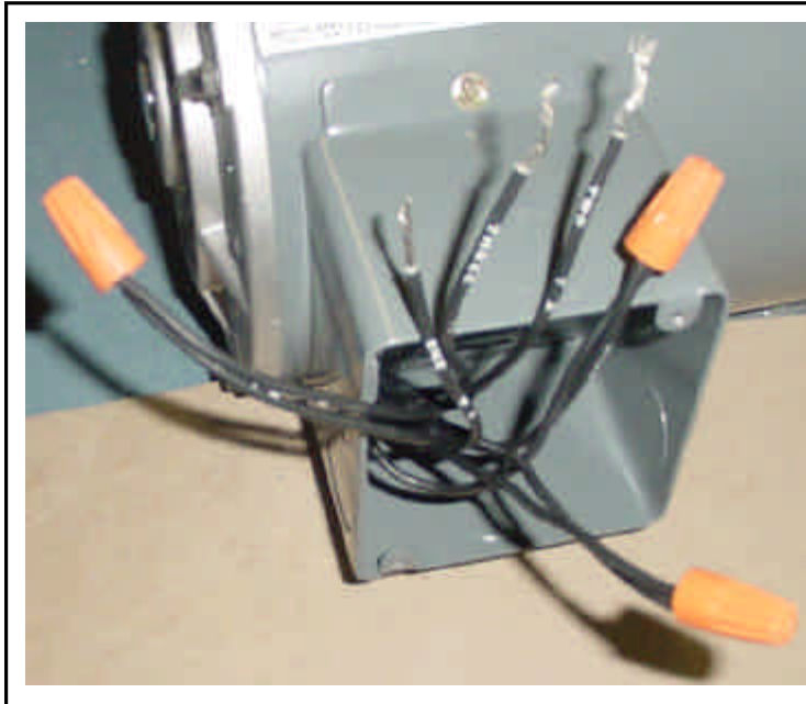
Wiring the LT1300300B for High Voltage (460v)
