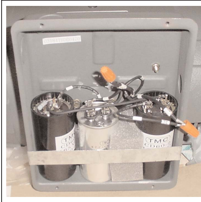
Wiring the LT2000500A for High Voltage (208-230v)
