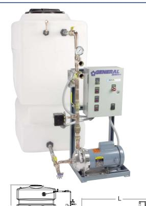
L x W x H OPS with 300 gal. tank: 93" x 36" x 57" OPS with 400 gal. tank: 93" x 36" x 71" General Air Products' Residential Fire Protection Pump System (RFP System) is the benchmark of quality for meeting 2010 NFPA 13D application requirements.
