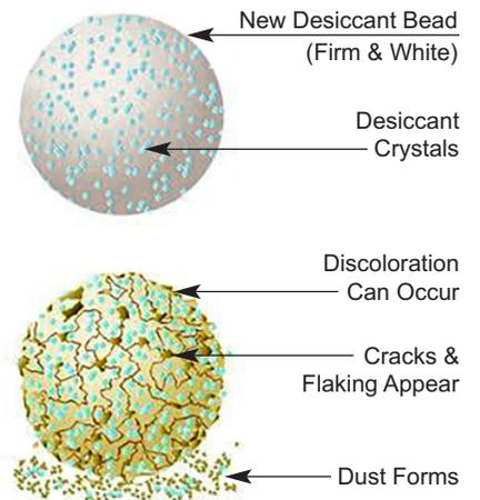
As the desiccant will degrade (age) slightly over time, it is recommended that the desiccant be inspected once every year. Desiccant beads should be firm and white with very little dust. Under normal operating conditions the desiccant should last at least 3 years. Replace desiccant sooner if any yellowing or powdery conditions exist.
