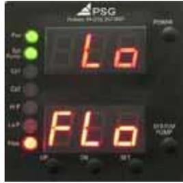
Water Flow: If the water flow drops below the point required to keep the flow switch closed, the “Lo Flow” alarm parameter name will flash on both numeric LED’s and the control will de-energize the compressors and hot gas valves. The re-circulation pump remains energized. It will reset automatically.
