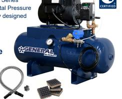
**New Digital Pressure Switch:** The ONLY UL Listed Digital Pressure Switch in the Fire Protection industry designed and built by the compressor manufacturer themselves. Displays Pressure Readings, Run Hours, Amps, Cycles, and is extremely easy to adjust pressure settings in the field. The Digital Pressure Swith also actuates an Automatic Drain Valve on tank mounted units.
