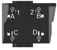
**1 & 2** - Use the rectangular holes on the bracket to rest it on the riser plate hooks.
