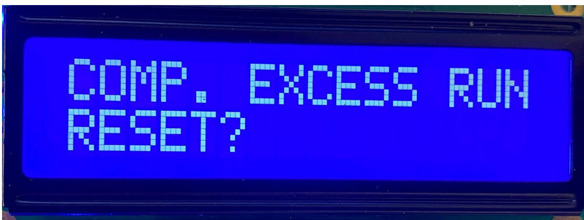
Figure 6. The alarm description is displayed when pressing "ENTER" with an active alarm.
