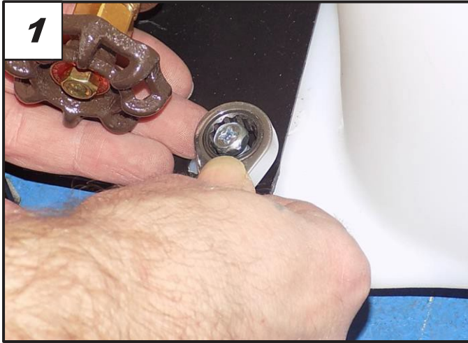
Remove the bolts on both sides of base plate.
